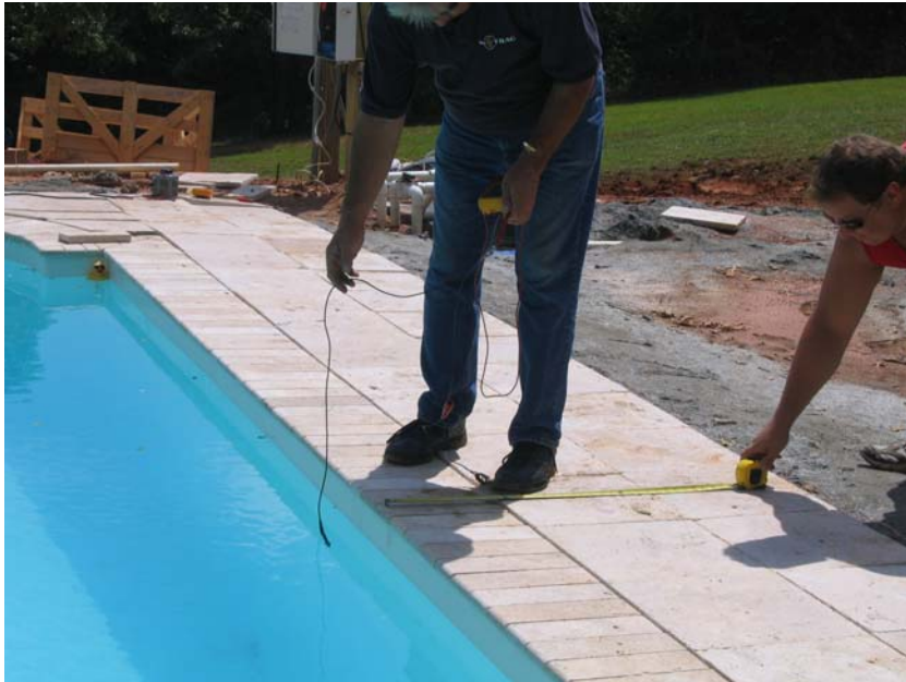
Figure 6: Typical Water-Deck Voltage Measurement
